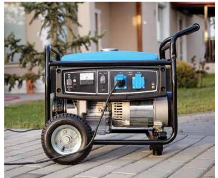
**#9 - Install a transfer switch.** A transfer switch connects the generator to the circuit panel and lets you power hardwired appliances. Most transfer switches also help avoid overload by displaying wattage usage levels.
